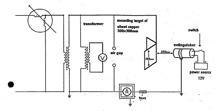
FIGURE 2. Test diagram for test 2: Electrical conductivity of FEAS fire extinguishing aerosol flow at the moment of discharge of the extinguisher.
