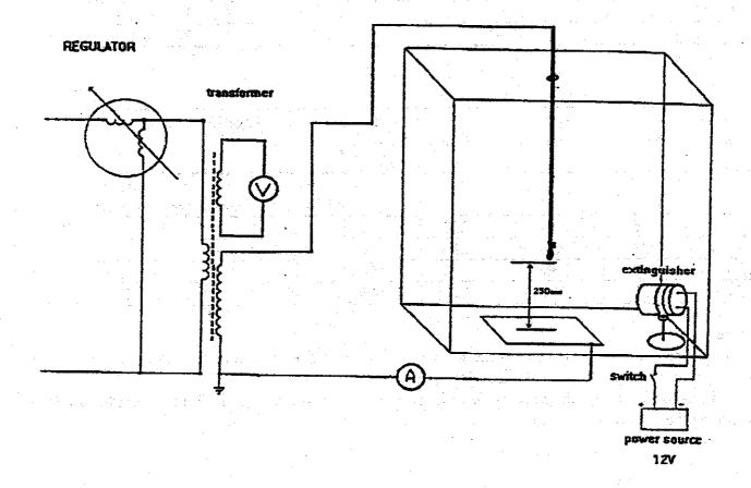
FIGURE 1. Test diagram for test 1: Electrical conductivity of FEAS fire extinguishing aerosol under total flooding conditions
